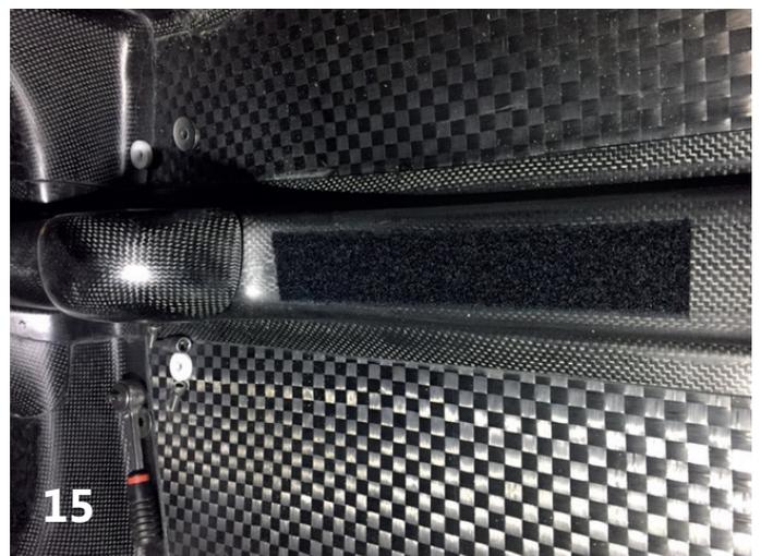
Photo 15: stick some Velcro (or other soft material) on the chain tunnel to avoid scratches and creaking sound.
