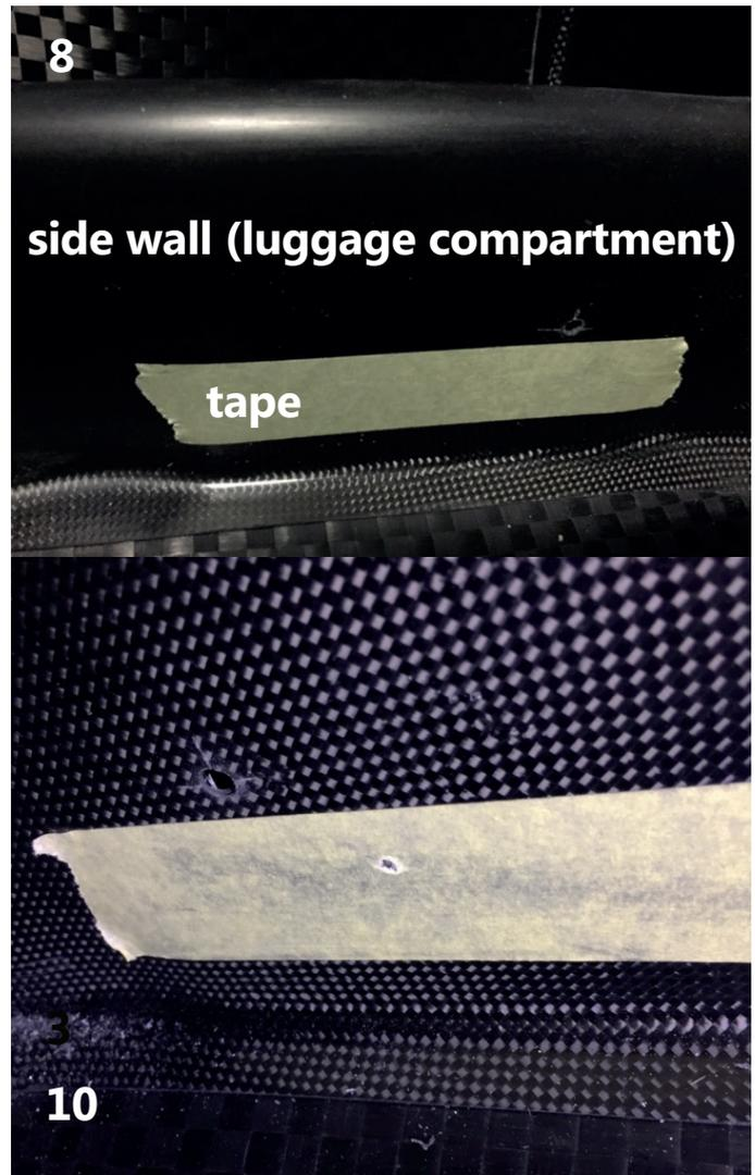
Put top and lower end of the seat in the desired position (pic 9). Make a mark on the tape with the bolts (pic 10). Check if both sides are marked on the same height from the bottom (pic 11).
