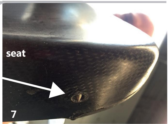
Screw in two (sharpened if possible) bolts into the bottom part of the seat from the inside (pic 6 and 7).
