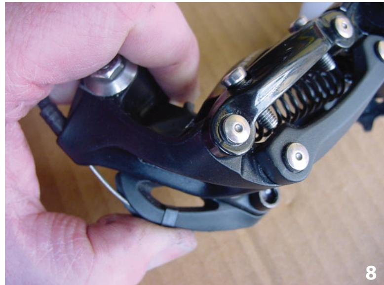
Move the derailleur to 11th gear while the cable slips underneath the bolt then tighten the bolt (pic 9).
