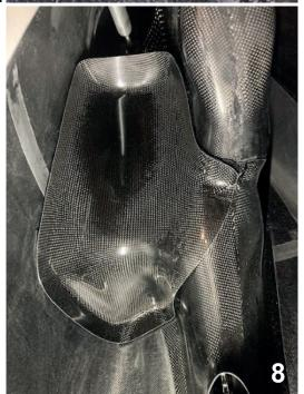
Pic 6 & 7) Remove the cover from your Snoek, remove the 5 velcro-loop parts and stick it along the masking tape in your velomobile.
