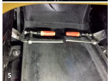
Use the clamps to secure the seat mounts in place (photos 4 and 5).
