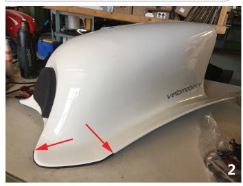
**Pic 1:** Remove old velcro on your QV (Quattrovelo) body: first heat it up little bit by hair dryer. No more than lukewarm, the paint and lamination of the body do not tolerate much heat! Then peel off the velcro, remove all glue rests.
