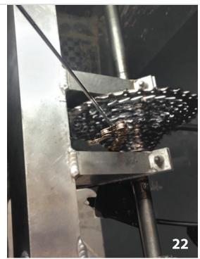
22. The tool in Photo 20 is also very helpful if the chain needs to be fished from the bottom after it was guided through the derailleur.
