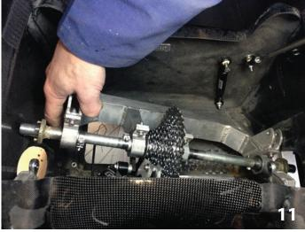
11. Rotate the assembly down while pushing the axle completely into its hole on the left side.
