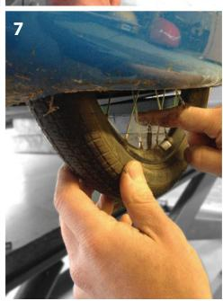
8. Slide the wheel of the axle, sometimes it needs a gentle knock with a hammer. If you only want to change the cassette you can slide the axles sideways after taking the wheels of.
