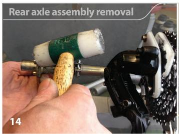
14. Tap on the axles to remove them from the cassette and bearings. Be careful not to bend the arms on the aluminum subframe.
