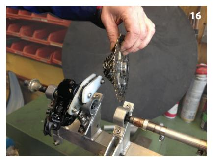
17. Note the position of the clamps and spacers. Older QV's have spacers of equal length most have spacers of different lengths.
