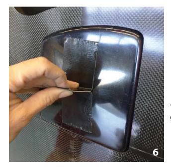
Stick the soft side of the Velcro to the dust and grease free sides of the new hatch and the other side to the body (fig 7).
