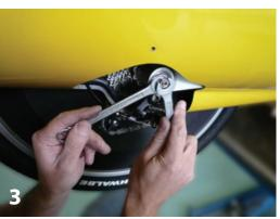
Loosen them using two 13 mm wrenches and remove them together with the thick washer.
