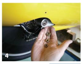
Then remove the M8 bolt with thick washer on the wheel side. If necessary, keep the shaft from turning with a 4mm Allen on the derailleur side.
