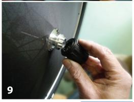
Thread the axle puller onto the end of the axle.
