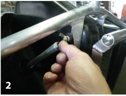
Two M8 nuts are locked against each other at the end of the axle on the derailleur side.
