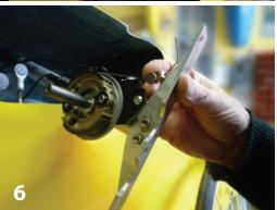
Loosen the two M8 (using two 13 mm wrenches) nuts that are tightened against each other on the strut assembly (thin nut on top) and remove the rubber ring and washer. (Picture 1)
