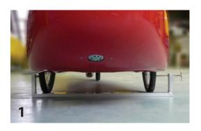
The alignment of the wheels is very important for the life of the tires and the performance of the bike. The front wheels should run exactly parallel. Measuring the toe-in accurately should be done on a flat surface.
