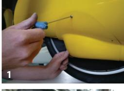
Set the derailleur in the 9th gear. This places it in a position to clear the body as the wheel moves down. Then disconnect the wing nut at the top of the shock and let the rear wheel drop.
